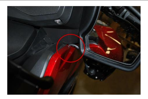
On the black portion of your plastics take a small rat tail file and remove just enough of the black plastic to not pinch the wire. Light mounting is complete.
