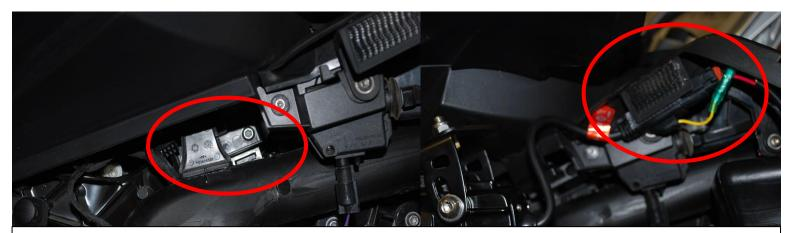
Remove the 2 factory bolts located on the inside of the side panel you can find these in the general area of the arrows above. Gently pull outward on the lower edges to release the posts from the rubber grommets. Once the posts are free gently pull the fairing back towards the rear of the bike and set side panel aside. (Note) you may need to disconnect electrical connections depending on model.
